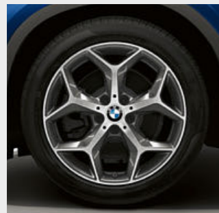
□ 18" light alloy wheels Y-spoke style 569, Orbit Grey, gloss-lathed, wheel size 7.5J x 18 with 225/50 R18 tyres.
