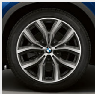
□ 19" light alloy wheels Y-spoke style 511 Orbit Grey, gloss-lathed with runflat tyres, wheel size 8J x 19 with 225/45 R19 tyres.
